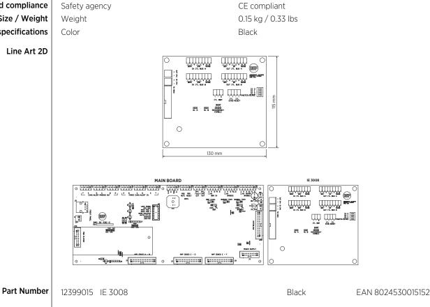
IE 3008 is an additional board for DXT 3000 system that extends its capability and functionalities allowing the connection of a maximum of 8 units, in a master/slave configuration. It shall be installed inside the cabinet of each device. System's units communicate through a redundant bus, transporting commands
