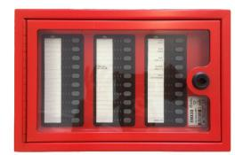
Top, bottom and rear cable entry points are provided by means of 'knock-outs' in the enclosure, while the field connections are provided by means of a set of terminals on the inside rear panel of the back box. The EMS10, EMS20 and EMS50 are compatible with the whole range of ASL Voice Alarm and Public Address systems, and are designed to comply with EN54-16, ISO 7240-16 and BS5839-8.
