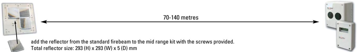
**140 - 160 metres - The standard 3000/FIREBEAM70 + 3000/FIREBEAM140/160 kit** - For distances of 140 to 160 metres you will need to use the standard firebeam and a long range extension kit (the long range kit comes with a backing plate and 8 extra reflectors, you will need to add the reflector from the standard kit to the long range kit with the screws provided)
