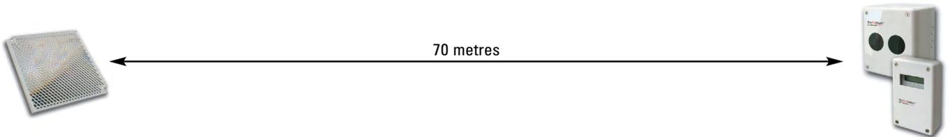
**70 - 140 metres - The standard 3000/FIREBEAM/70 + mid range 3000/FIREBEAM70/140 kit** - For distances of 70 to 140 metres you will need to use the standard firebeam and a mid range extension kit (the mid range kit comes with a backing plate and 3 extra reflectors, you will need to add the reflector from the standard kit to the mid range kit with the screws provided)
