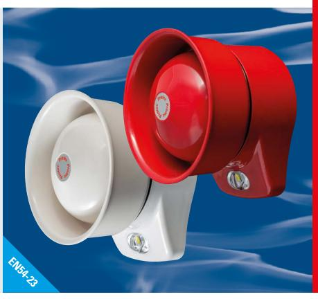
The Protec 6000/TSR/VAD is a loop driven, addressable high intensity Visual Alarm Device (VAD) with up to 7m room coverage and a high output electronic sounder with up to 100dB(A) at 1m. Combining the two functions in one compact high efficiency design improves the aesthetic appearance and simplifies the installation of the device.
