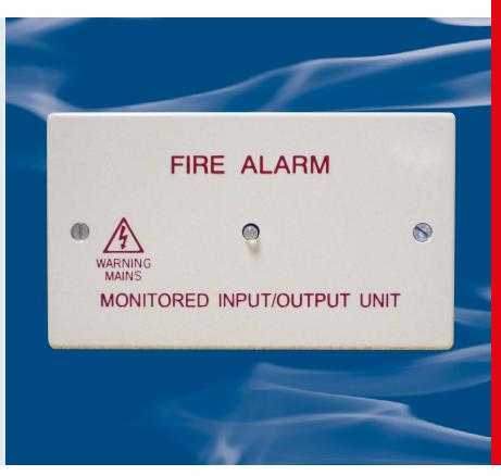
The Protec 6000 series MICCO is a loop powered fault monitored input and a volt free clean contact output interface. An on board isolator is provided which protects against loop short circuits on either the incoming or outgoing loop connections.
