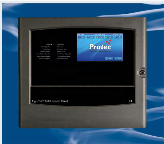
The Protec 6500 repeat panel can be connected to the secure local network. The repeat panel has an identical display to the control panel including a full colour 7" touch screen graphical display, zonal fire LED's and system LED's for information purposes and mandatory functions. The repeat panel is available as surface or recessed mounted with a moulded polycarbonate hinged door finished in storm grey.
