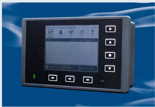
The 6000/LOOP/REPEATER can be connected directly to the local Algo-Tec™ digital addressable data loop and takes up just one address. Events from the main panel are displayed on the repeater's large LCD display, providing system indication of any loop connected location on site. The low power consumption allows numerous repeat devices to be fitted, greatly increasing system visibility.
